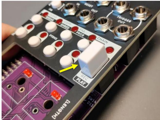
Flip the module over and make sure it rests on the cap of the toggle switch.
