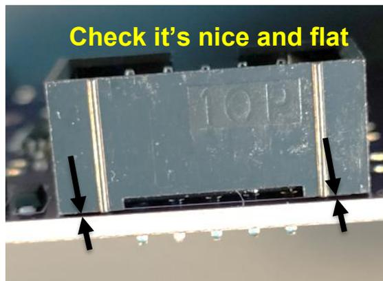
Once the power connector is sitting nicely, solder all the remaining pins.
