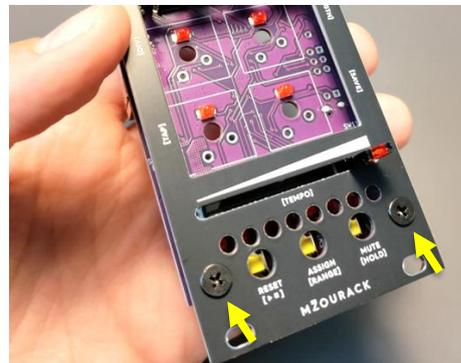
Attach the nuts to the two outer-most jack sockets.
